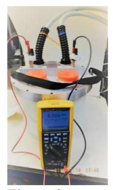
Figure 2. Meter indicate 6.02 volts= 60.2 kv applied. Actual applied was 60.175 kv
