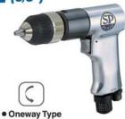
Chuck Size : 3/8" Free Speed : 2,500 rpm Overall Length : 6-3/4" Net Weight : 2.1 lbs. Vibration Level : 0.4 m/s2 Sound Level : 84 dB
