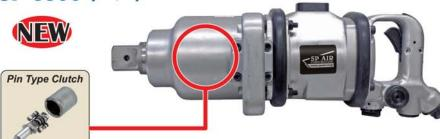
: 1-1/2" Sq.Drive : 2-3/16" **Bolt Capacity** Max. Torque Range: 3,000 ft-lbs. Free Speed : 3,600 rpm Overall Length : 21-3/4" Net Weight : 39.9 lbs. Vibration Level : 9.3 m/s2 Sound Level : 107 dB
