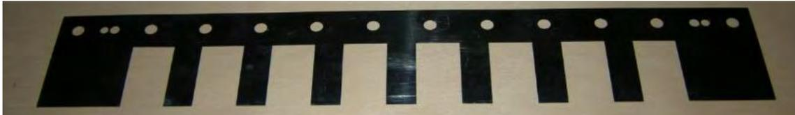
... are made by appropriate shims, lasercut from steel or kapton
