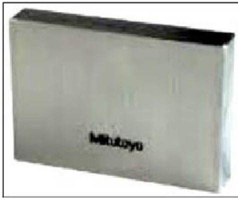
Gauge Block. The long dimension is two inches.
