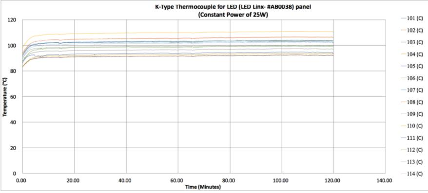
Within twenty minutes, temperature on the average varied from 90C to about 110C for various thermocouples
