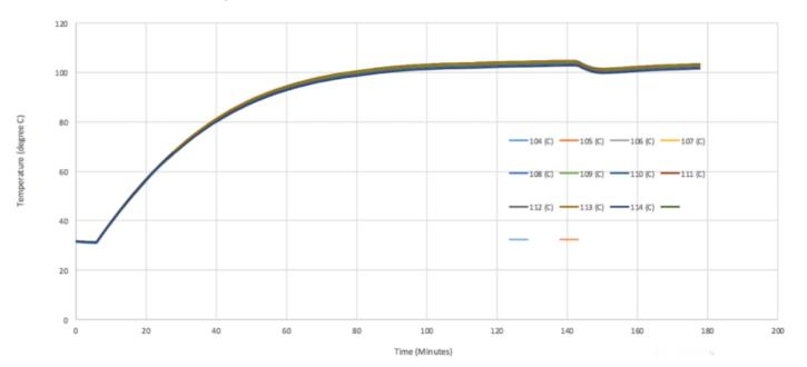
A base plate was used to mount the LED panel and in this case, all thermocouples collectively reached to an average temperature of about 92.1 C as shown
