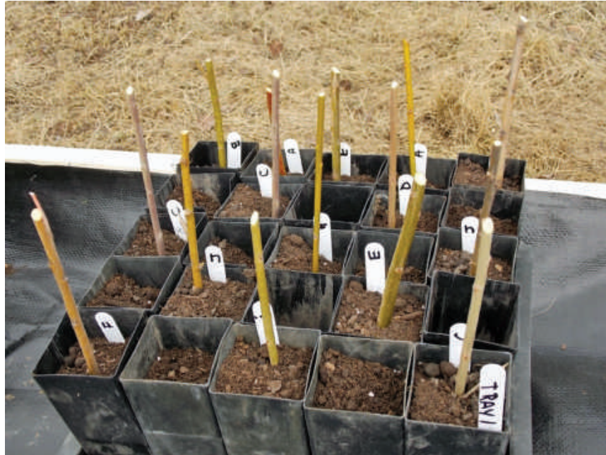
FIGURE 2. Set up of blind bench/field trial comparing treatment of and tolerance to petroleum hydrocarbon contamination between different hybrid and native willow clones. The bench/field approach was used to combine the controls of a bench study with containers, in a long term (two year) field setting.
