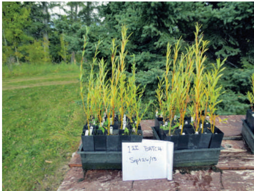
FIGURE 3. Results show no phytotoxicity at 20,000 ppm TPH (total petroleum hydrocarbon) after five months.
