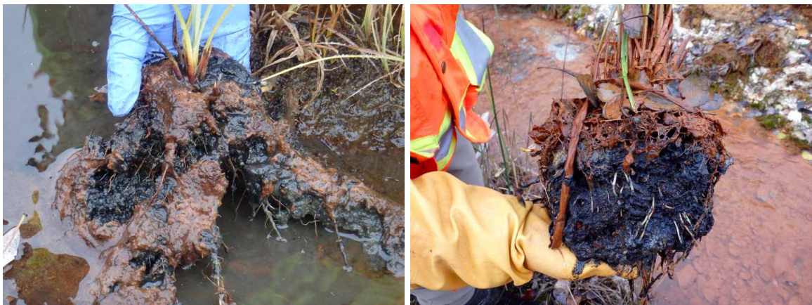
FIGURE 4. Examples of redox conditions that exist around plant roots within a wetland. Black is indicative of sulphate-reduction and a negative redox, while the red is indicative of oxidized iron and a positive redox. Over time and with accretion, the red/oxidized regions can be sequestered into the sediment as reduced sulphidic minerals. This natural cycle must be considered in PWTS designs incorporating plants.
