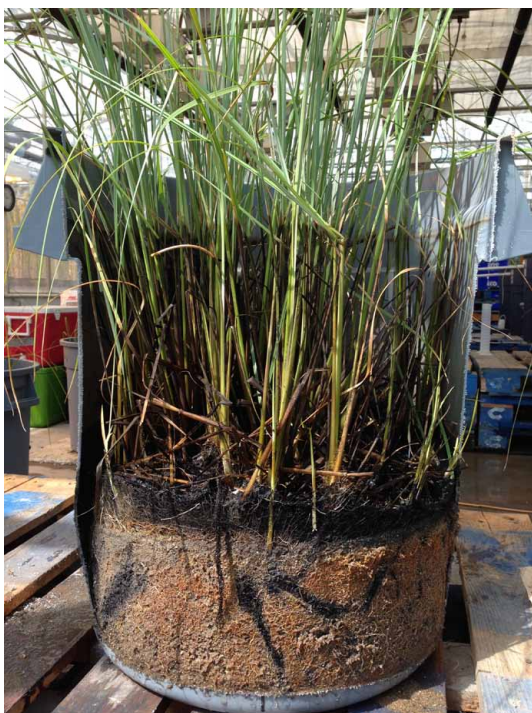
FIGURE 5. Pilot-scale PWTs cell constructed for copper and selenium treatment for the Minto Mine, Yukon Territory. Pilot system dismantling with plants exhibiting relatively low ROL. Regions of sulphate reduction are found at the sediment/water interface and in the root zone (black areas). In this system, copper treatment was highly correlated to sulphur deposition in soils and not correlated to iron concentrations.
