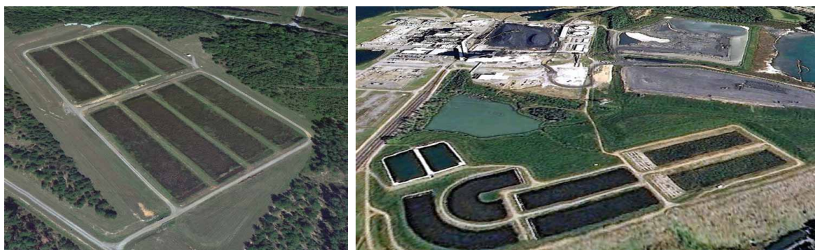
FIGURE 10. Full-scale PWTS. Left, Savannah River Site A-01 (South Carolina) has been in operation since 2000 treating for copper, zinc, and mercury (Nelson 2010). Right, PWTS treating flue gas desulfurization waters (Eggert et al., 2008; Dorman et al. 2009).
