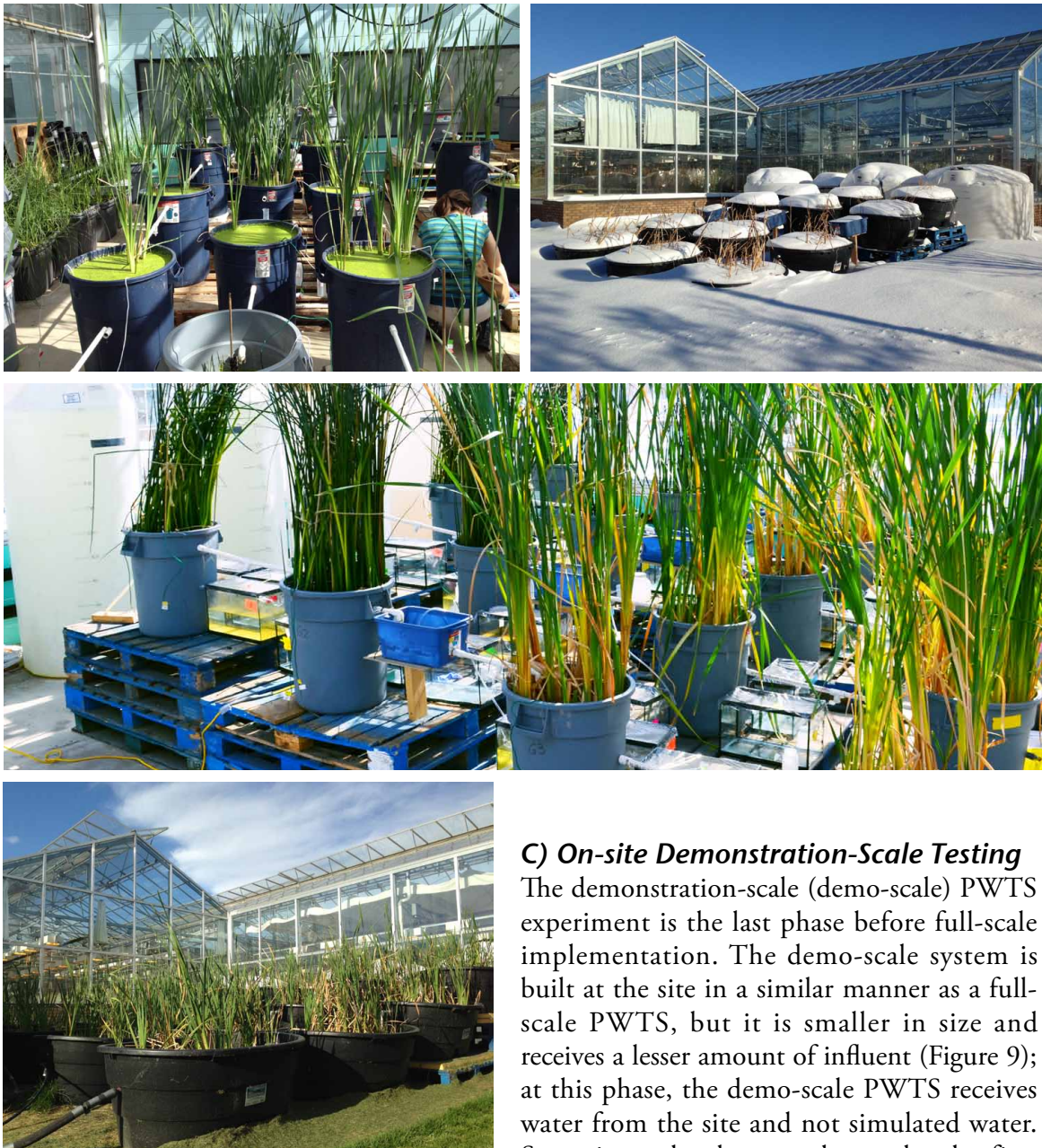
FIGURE 8. Examples of pilot-scale PWTS testing in a controlled indoor (top left and middle figures) and outdoor (top right and bottom figures) setting.
