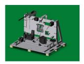
Project: End Of Line Test Station / Customer Interface Gage Notes: Tool test part, verifies correct assembly and gages interface with customers part.
